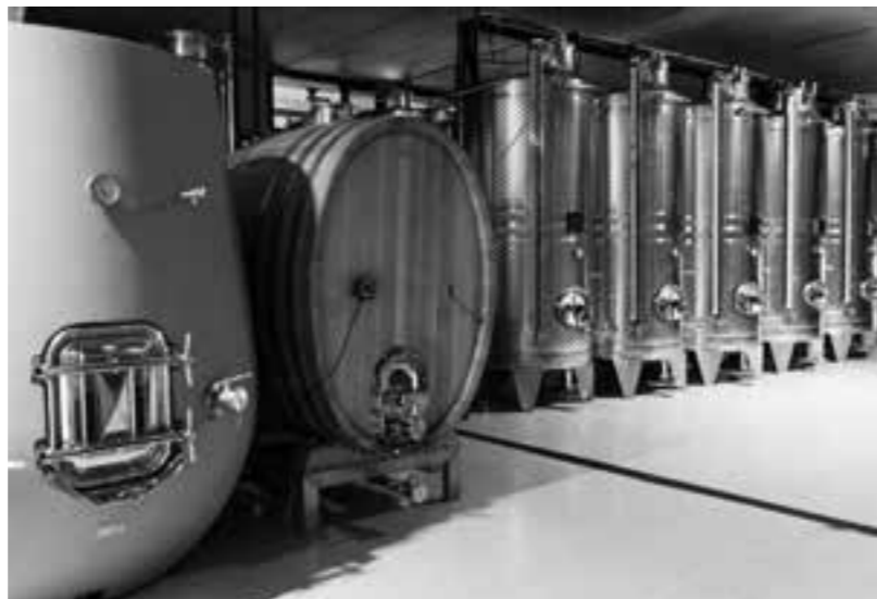
Stainless steel, wooden and concrete vessels coexist at Oenops Winery, reflecting a philosophy that embraces multiple winemaking techniques.
